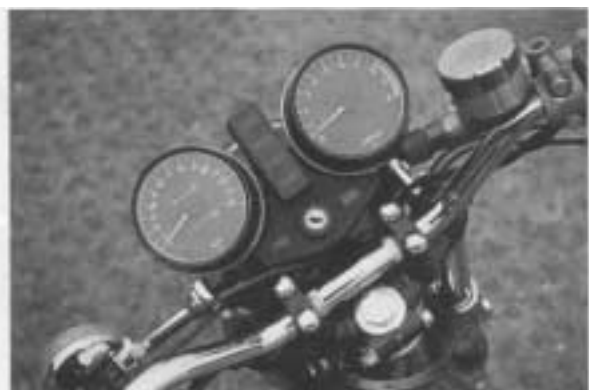
A Redline starts just before 8000rpm, but engine can be safely spun to the end of the dial. Three figure speeds are easily reached
